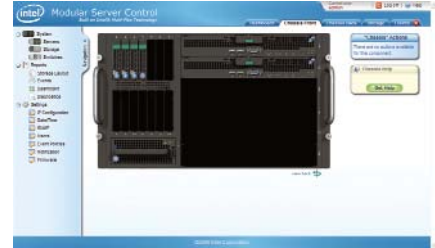
The Virtual Presence Modular Server Control allows you to see the components you physically have loaded in your system—even if they are powered down
