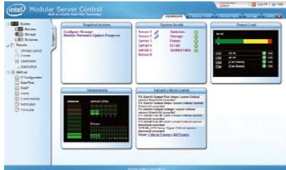
The Dashboard gives an overall system status view within the Modular Server Control
